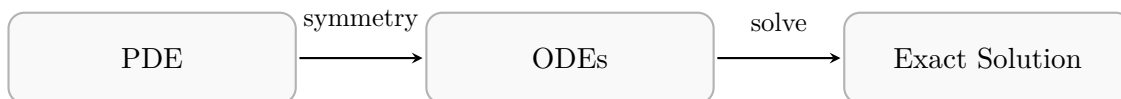
Figure 3.2: Lie symmetries are one way to reduce a PDE to a set of ODEs.
